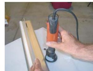
A Rotary Tool Cutting Adapter is perfect for clean, easy to make, grooves for Fiber Carbon rod wing spar. Glue spar in with RC Z 56 or medium/thick CA.
