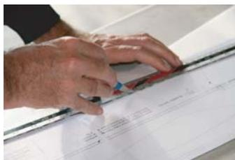
Carefully cut each out using a straightedge and #11 Xacto.
