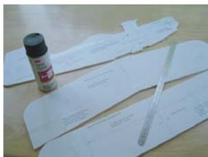
Lightly coat back of plan parts with Spray Adhesive, apply each part to Depron. Carefully cut each out using a straightedge and #11 Xacto.
